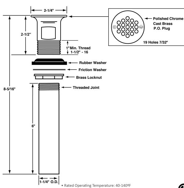
• Note: 180°F max. during temporary high-temperature system flush
